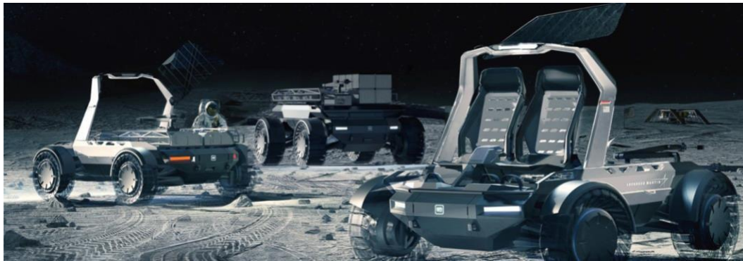
Figure 1. The Lockheed Martin Lunar Mobility Vehicle (LMV) enables unprecedented exploration of the Moon with autonomous, telerobotic, and manual operation. Credit: Lockheed Martin. 1
